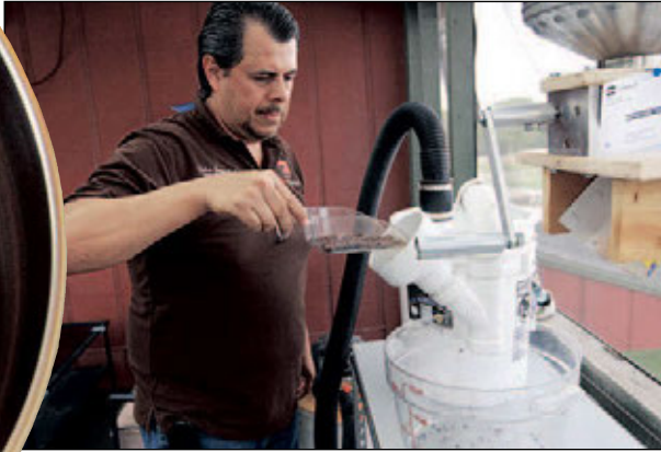
Benavidez uses a machine he created to separate cacao shells from their useful interior after they have been ground into chunks.
